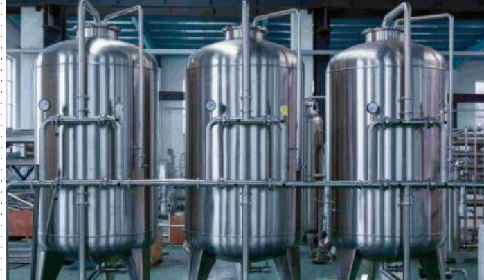
Filter system for mechanical water purification
